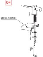
Place faucet body through the hole of basin countertops. Pad the rubber washer and locking washer in order. Tighten them with locking nuts.
